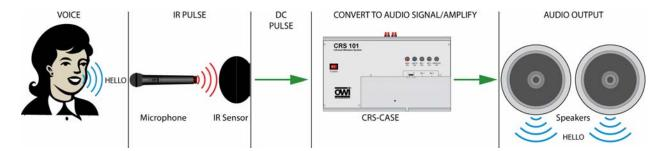
Figure 15. CRS-101 System Signal Path
